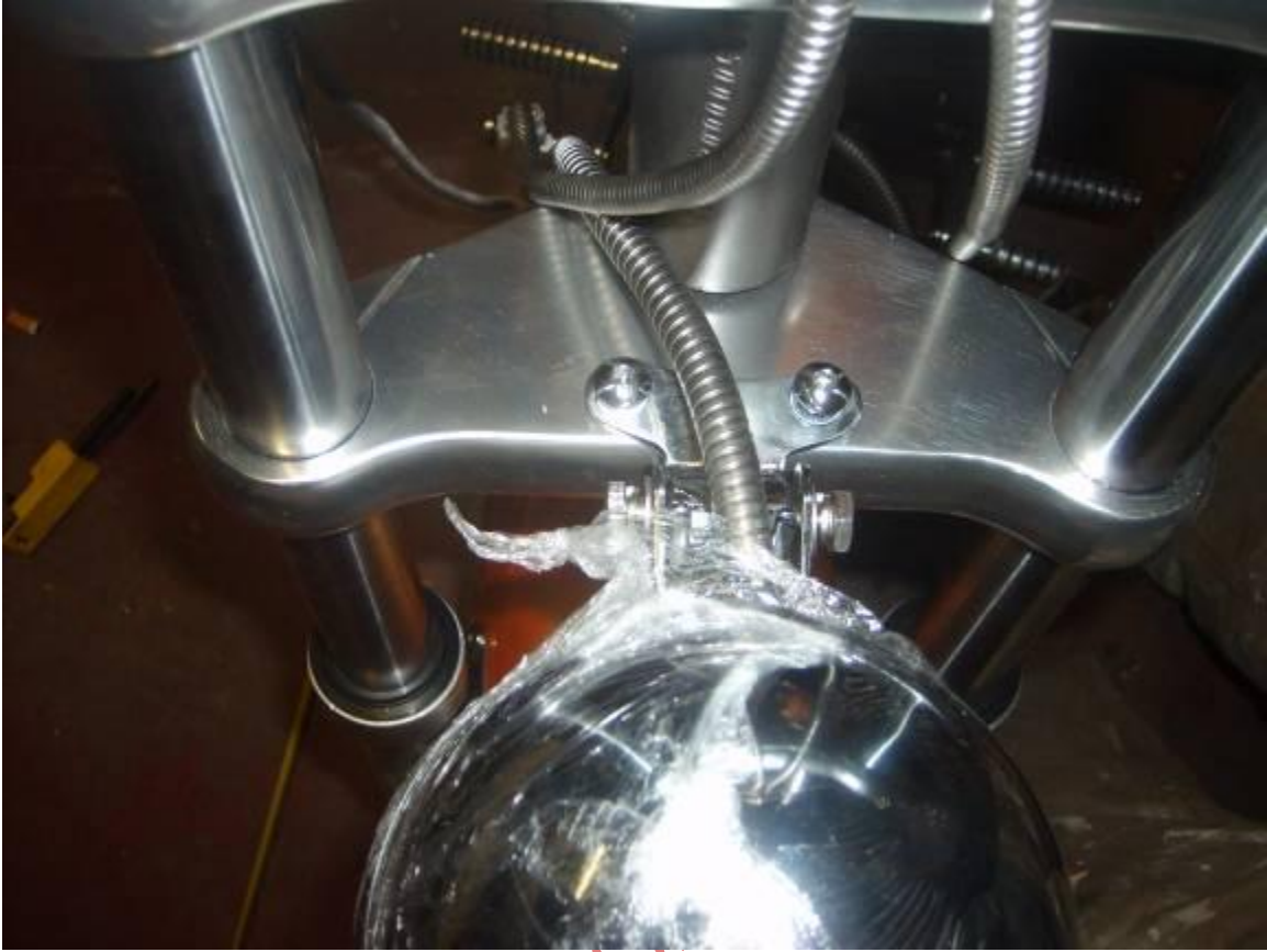
The head light plugs into the corresponding plug under the tank.
