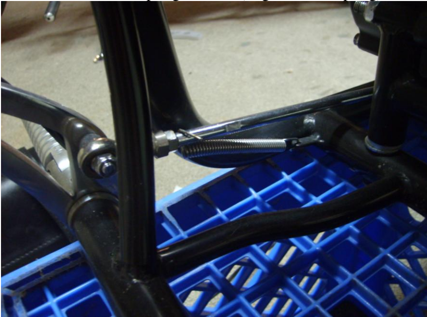
Rear brake accuator spring location
