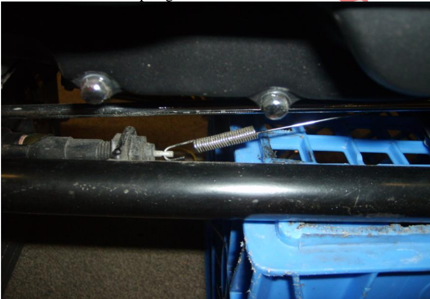
Rear brake accuator spring location
